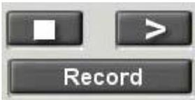
With these buttons the Project can be played or stopped or have a recording made by touching the “Record” button. Remember that one of the Tracks must be selected to Record before you can use the “Record” button here.
