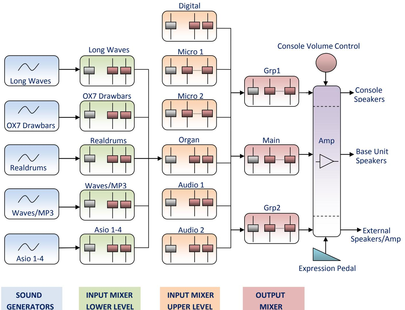
On the input mixer most of the equalisers comprise just a **Bass** and a **Treble** control, the exception being those on the external microphone inputs **Micro 1** and **Micro 2** which have the full four band **Bass, Mid 1, Mid 2** and **Treble** controls. On the Output Mixer all equalisers have the full four band controls.
