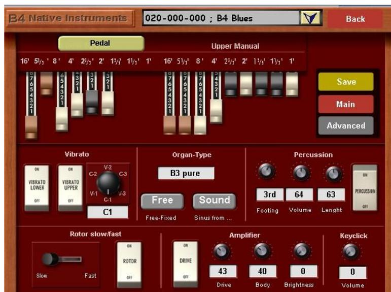
This screen provides a simulation of the controls of the **Hammond B3 organ**. As yet we have had no articles on our website explaining how to use this editing feature. It does enable you to produce User B4 Sounds by adjusting the controls on this screen (**Main**) and the **Advanced** controls which replace the lower half of the display when the Advanced button is touched.
